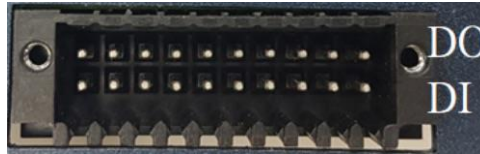
2.54mm 2x10 Terminal Block Including (DI: 8bit, DO: 8bit, 3.3V Power and GND pins).
